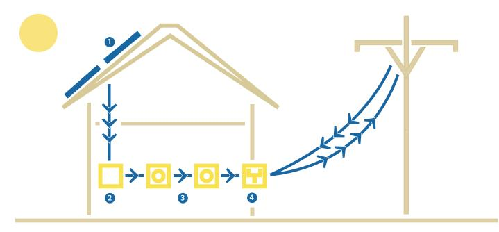
Solar PV systems capture sunlight and convert it into electricity that can be used to power your home or business. Basic grid-tied solar systems consist of solar panels, inverters, racking, meters and disconnect switches. Optional components include monitoring systems and batteries.
