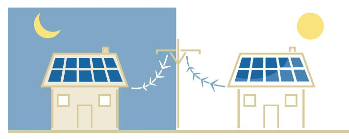
Production from a PV system rises and falls with the sun. During the night when solar panels aren't generating, you're meeting your power needs by drawing electricity from the grid. During the day, as electricity production increases, there may be times when your system produces more than enough electricity to meet your needs and excess power is sent onto the grid. Either way, a grid-tied solar system uses the grid 24 hours per day.
